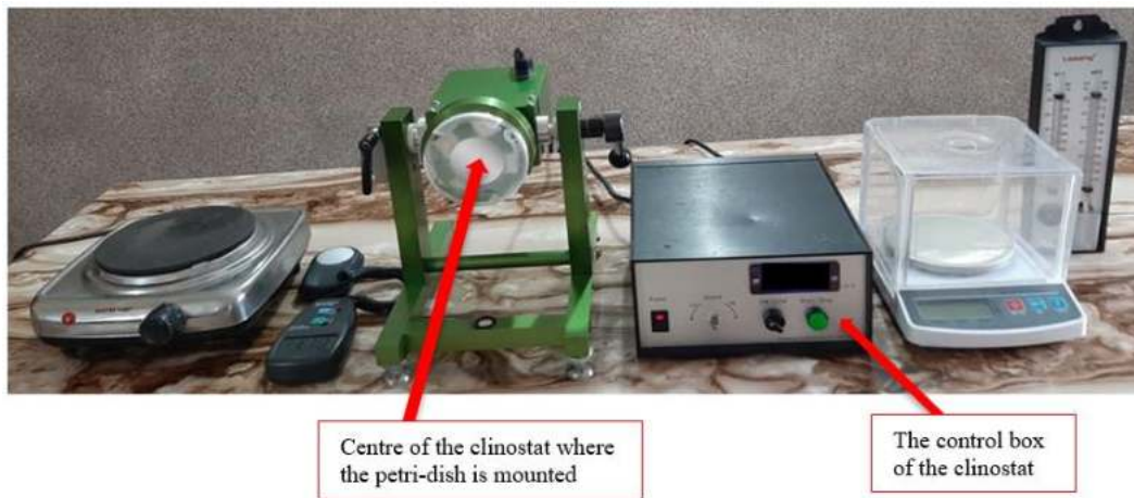
Figure 2. Experimental set-up for clinostat use
